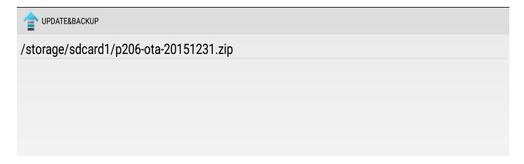
5. Then press update: device reboot and start installing firmware. Do not power off device during installing.
